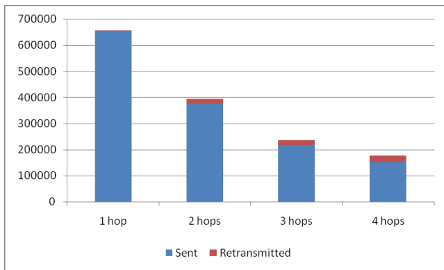
Figure 5. Bytes/s transmitted in different number of hops
